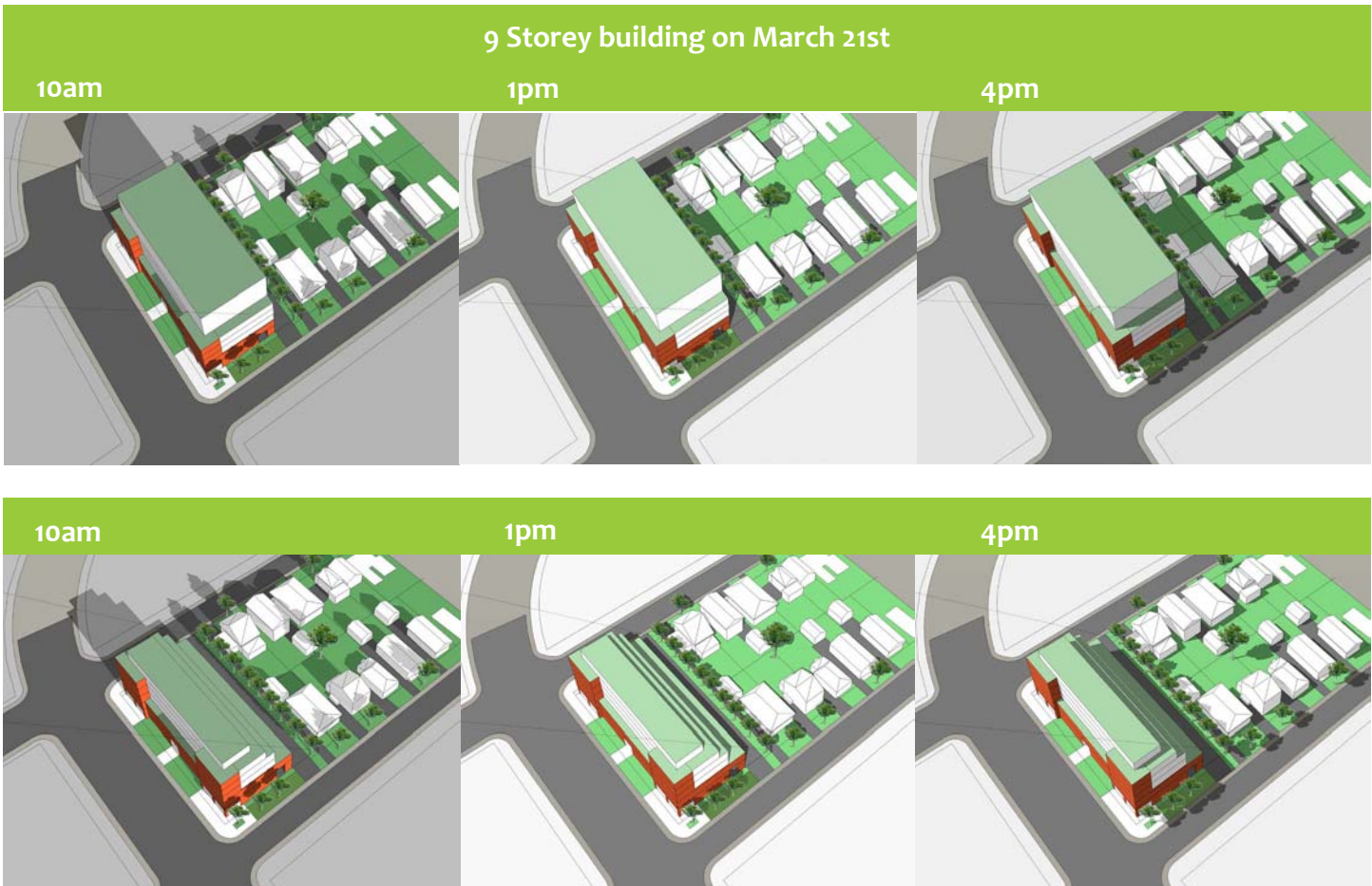
Building height reduced and designed with upper floor terracing and setbacks to minimize shadows on adjacent properties
